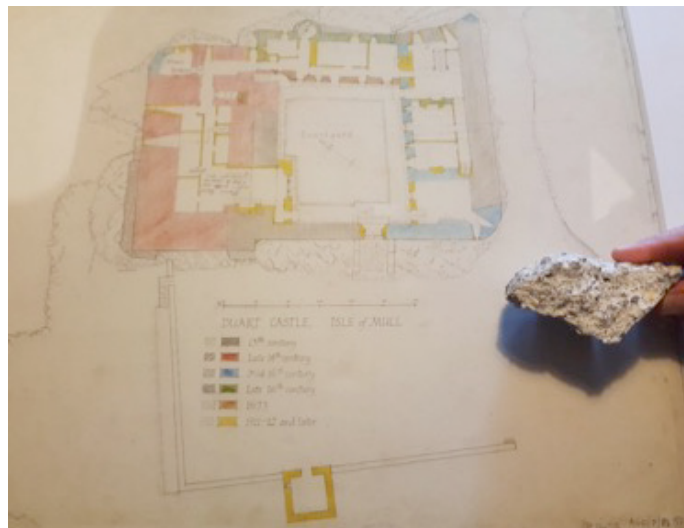
A plan showing the chronology of Duart Castle, and a piece of early mortar which is being matched in a hot mix in the current work. Some of the walls are 5 metres thick. Photo Nicola Ashurst
